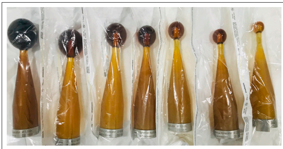
FIG 2. IORT Intrabeam 50kV, Carl Zeiss Surgical, Oberkochen, Germany applicators ball types.
