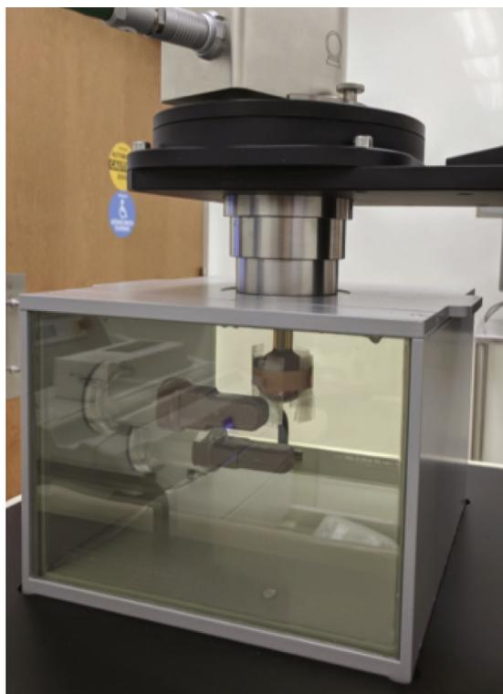
Fig. 1. The in air OSLD calibration measurement setup is depicted with four OSLD chips placed 90° apart on the surface of an INTRABEAM spherical treatment applicator. OSLD = optically stimulated luminescence dosimeter.
