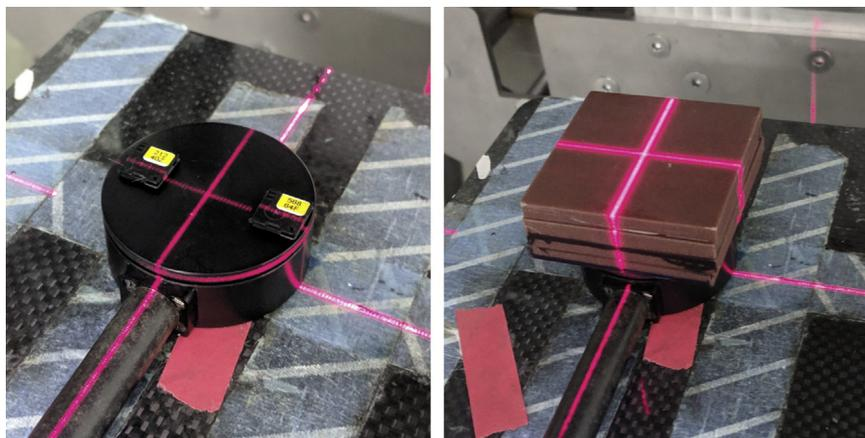
Fig. 2. The energy dependence measurements related to beam hardening are shown with the parallel-plate ion chamber and OSLD chips placed as illustrated, with solid water blocks added to simulate varying tissue depth. OSLD = optically stimulated luminescence dosimeter.
